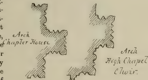
FIG. 1000.—Iona Cathedral. Section of Arch Mouldings.
